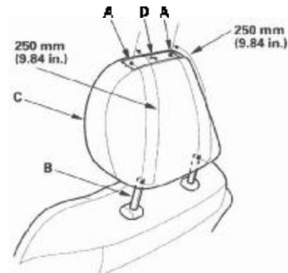
6. Push the head restraint (A) forward, and check: With a ruler, measure the level amount of the head restraint movement. The head restraint should move more than 50 mm (2.0 in.) without resistance. If it is less than 50 mm (2.0 in.), or the head restraint doesn't move smoothly, replace the seat-back frame assembly:
