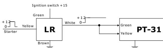
Additional so called locking relay LR is available for diesel cars. It is connected between the starter terminal in ignition switch and the input (yellow and green wires) of the automatic relay PT-31.
